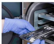
*Autoclave sterilization works by using high heat (250°F+) to kill microorganisms such as bacteria and spores. Heat is delivered by pressurized steam that allows the high temperatures required for sterilization. GOEX extrudes Polycarbonate and Polypropylene options that withstand this form of sterilization.*
