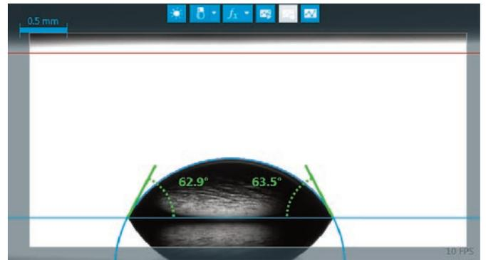
contact angle meter to understand surface treatment better, and if possible correlate contact angles to dyne results as a means to validate our dyne measurement process.
